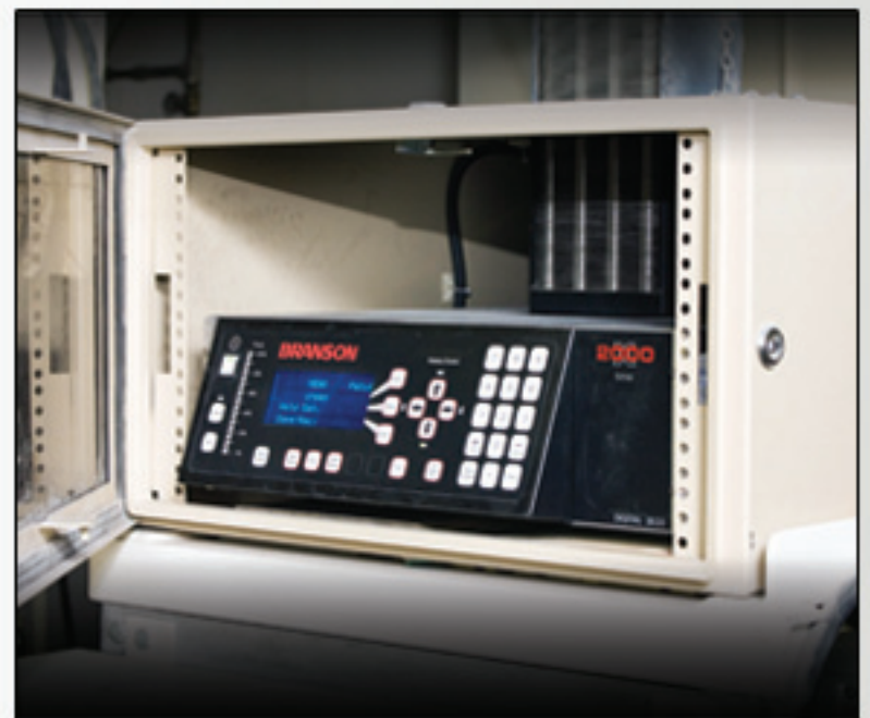
2000XT power supply which fits into the existing enclosure
