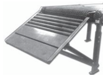
Roller Discharge with Stop Plates
